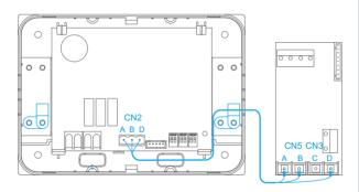
Wiring method 2: Lay the communication wire through the hole on the base of the refrigerant leakage alarm to terminals A and B of CN5 and terminal D of CN3 on the IDU extension board. Fix the wire to the base with a cable tie to avoid placing stress on the terminals.
