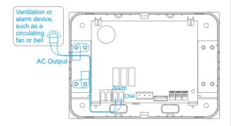
Wiring method 2: Lay the cable through the hole on the base of the refrigerant leakage alarm to the terminals of CN4, and fix the cable to the base with a cable tie to avoid stress on the terminals. Connect the other end of the cable to the power input end of a ventilation or alarm device.
