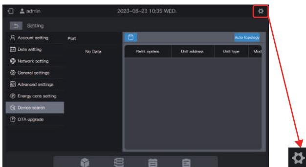
Click "Device search" in the left menu and "Auto topology" in the right area. The centralized controller will start to obtain information about the refrigerant system connected to the centralized controller and automatically construct the topological relationship. After this, the interface will appear as follows:
