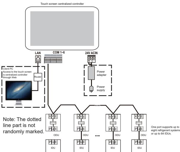
Note: There may not be a PQE interface between an IDU and an ODU. For details, refer to the manual of ODU and IDU. This is only used to illustrate the centralized controller framework.
