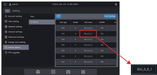
**Mode 2:** Modify the unit name on the "Device monitoring" interface.
