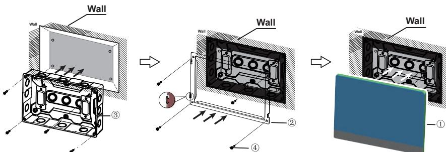
Attention: The controller is only suitable for installation at a height of  $\leq 2\text{m}$ .
