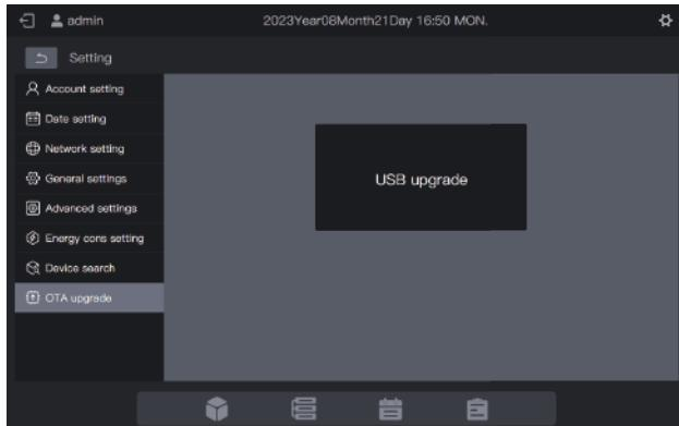
Click "OTA upgrade" and select the package to be upgraded in the pop-up interface. The centralized controller will automatically restart and upgrade the firmware.
