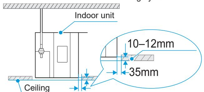
**A** After adjusting the indoor unit position and level, tighten the nuts on the mounting hook to secure the air conditioner in place.
