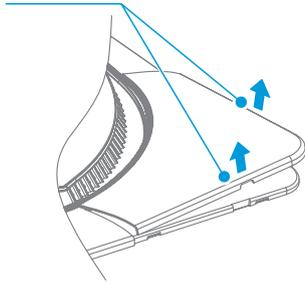
3 Loosen the locking screws at four corners and remove the hooks at four corners of the panel from the indoor unit.
