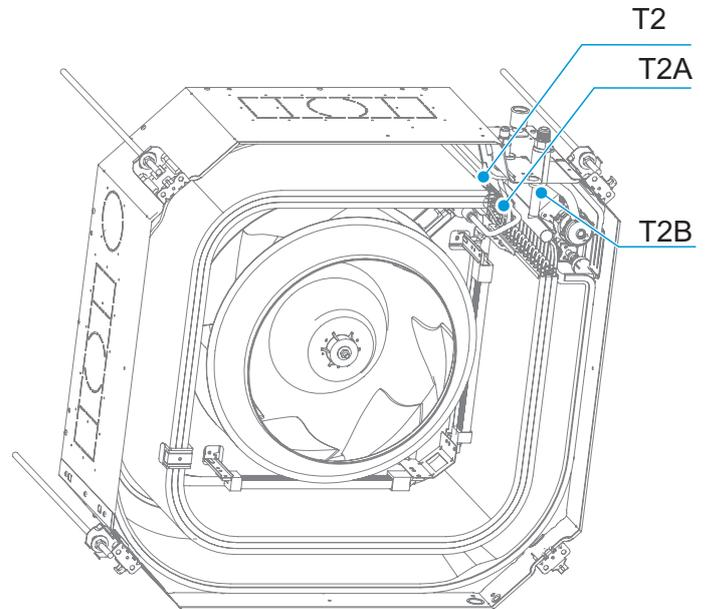
**8** Remove the connecting pipes of indoor unit and outdoor unit and unscrew the two screws of the sealing plate of the piping to remove the plate.
