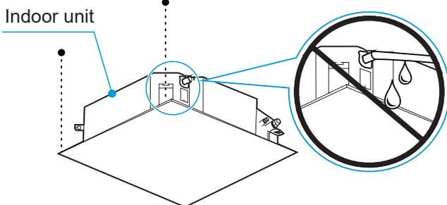
**B** Adjust the position of the indoor unit to ensure that the interval of the four sides of the ceiling is even, and the bottom surface of the indoor unit should be recessed from the bottom surface of the ceiling by 10-12mm.
