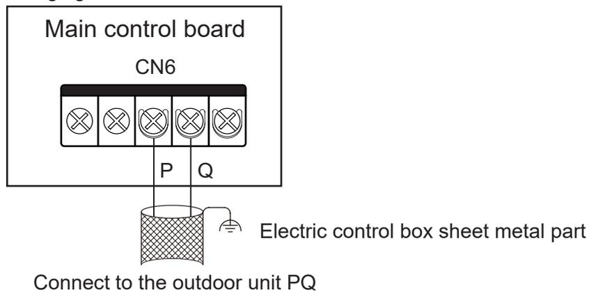
System: The maximum total length of the P/Q communication cable of the Indoor unit and outdoor unit can be up to 1200m, and can be connected in serial, as shown in the figure below:
