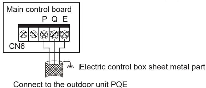
System: The maximum total length of the P/Q/E communication cable of the indoor unit and outdoor unit can be up to 1200m, and can be connected in serial, as shown in the figure below:
