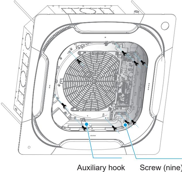
3 Remove the nuts with flat washers and the fan clip at the position shown in the figure, and remove the fan.
