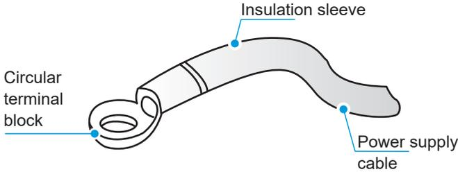
**C** If it fails to crimp the insulated circular terminal block due to on-site limitations, connect the power supply cable of the same diameter to both sides of the power supply terminal block of the indoor unit, as shown in the figure below.
