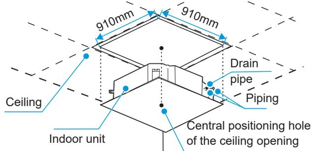
Using a pencil, mark the positions on the ceiling slab where the suspension bolts need to be fixed based on the distance between the four hanging holes on the indoor unit.
