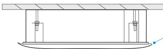
NOTE: Without support from the ceiling, tightening the screws too much will deform the panel.
