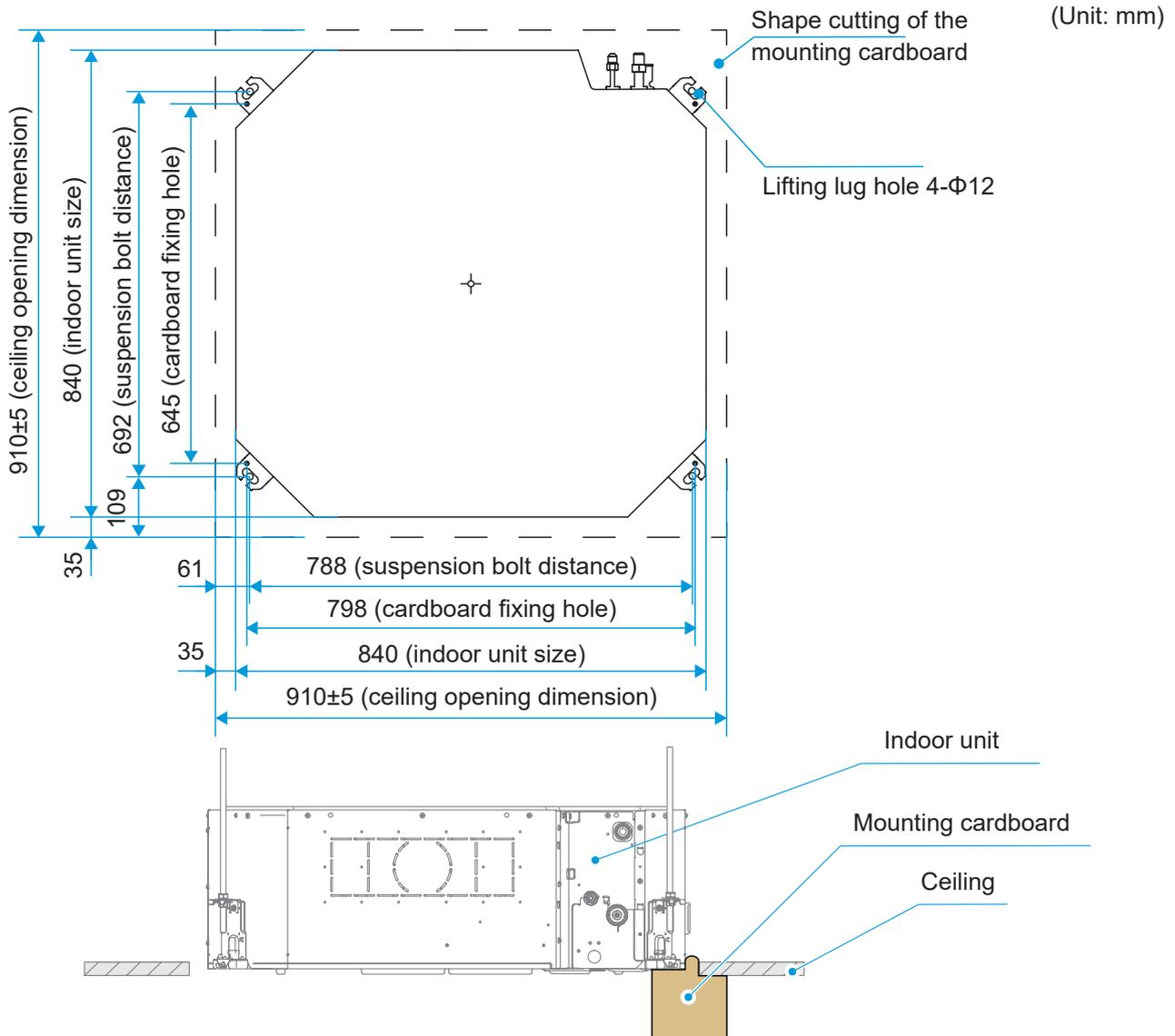
The mounting cardboard is used to adjust the distance between the indoor unit and the ceiling to ensure that the panel fits closely with the ceiling after installation.
