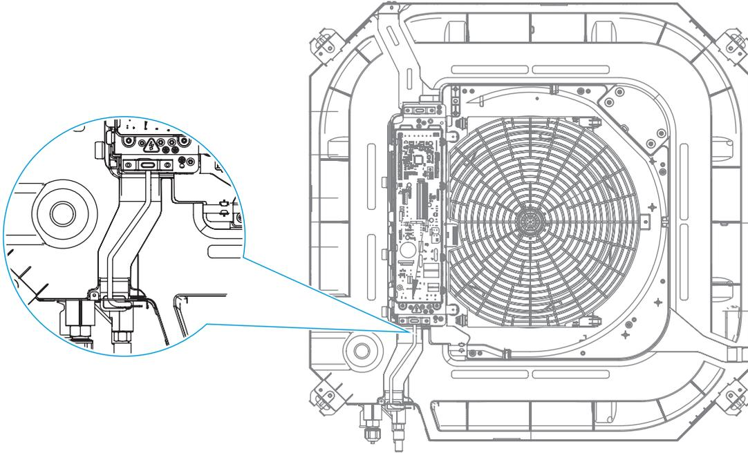
Route the power cord, ensuring that it has a certain degree of slackness. Remove the screw of the sealing plate, use the accessory cable clamp to clamp the power cord, and then use the screw to fix the cable clamp on the sealing plate.
