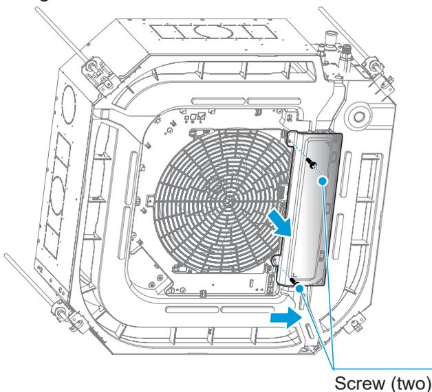
3 Remove the electric control board.
