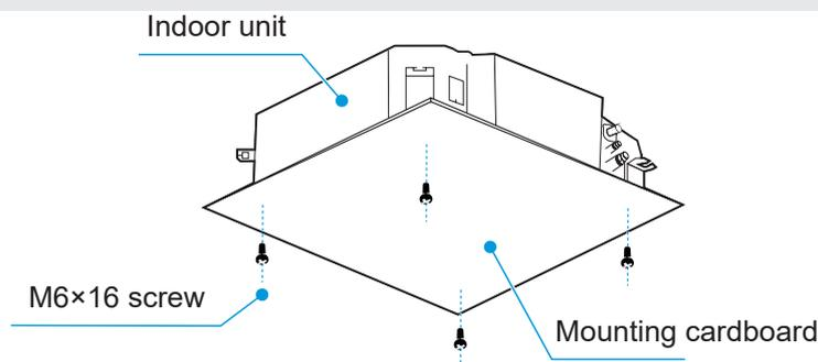
③ Carry out installation as described above (Point 3 of Existing Ceiling installation).
