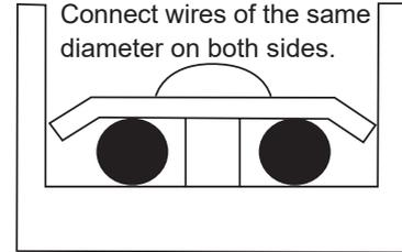
**D** Do not press the power supply cable of the same wire diameter on the same side. Do not use two power supply cable of different wire diameters for the same terminal blocks; otherwise, they can easily loosen due to uneven pressure and cause accidents, as shown in the figure below.
