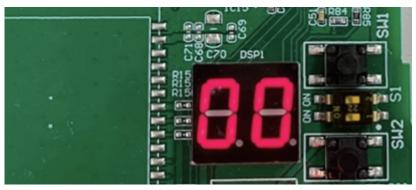
Once powered on, the digital display shows the software version. After the software runs properly, the numbers of IDUs and ODUs are displayed alternately.
