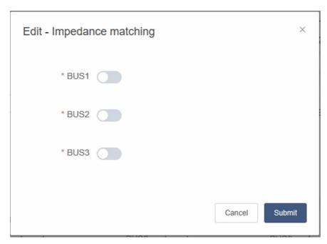
This pane displays the status of impedance matching. You can click "Edit" to enable or disable impedance matching for buses.
