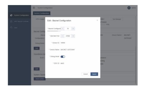
2.1.2 Check whether the BACnet function of the Gateway is normal on the **VRF Bacnet Console** page.
