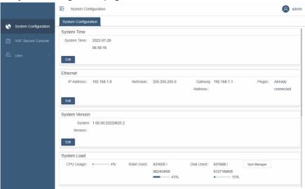
2.1.1.1 Open the System Configuration page, and click "Edit" in the **Ethernet** pane, and edit relevant parameters in the opened dialog box.
