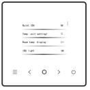
After the IDU light is enabled, the IDU display LED will light up. After the IDU light is disabled, the IDU display LED will turn off. You can press "  $\bigcirc$  " to turn on or off the IDU light.
