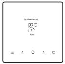
Select the swing (left/right) up/down function on the menu, and press "  $\bigcirc$  " for confirmation. After entering the swing interface, press " < " or " > " to adjust the swing angle, or press "  $\equiv$  " to return to the menu.
