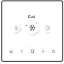
Select the mode on the menu and press " \( \) " for confirmation. After entering the mode, press " < " or " > " to select the operating mode. and press "  $\cap$  " for confirmation. Or press " = " to exit. Mode conflict: When the system detects any mode conflict, the main screen of the wired controller will display a message indicating that
