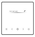
Select the setting on the menu, and press "  $\bigcirc$  " for confirmation. After entering the function setting interface, press " < " or " > " to switch the function, and press "  $\bigcirc$  " to enable the selected function.
