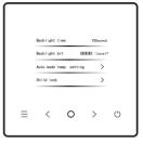
The backlight brightness has 10 levels, used to set the display brightness of the device. The brightness increases from level 1 to 10. You can press "  $\bigcirc$  " to adjust the backlight brightness.
