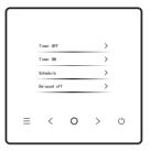
Select the timer function on the menu, and press " \( \cap \)" for confirmation. After entering the timer interface, press " < " or " > " to select the corresponding timer. and press " \( \) " to start function setting.
