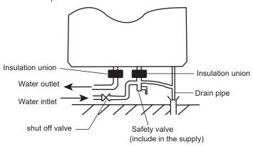
Depending on the degree of humidity in the air you can get up to 0,25l/h of condensation. The evacuation of condensate should not been made directly to sew water because of possible corrosive gasses damaging the exchanger fins and water heater parts.
