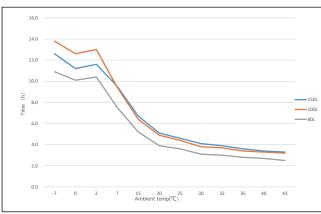
When ambient temp below 2°C, heat pump and E-heater will take different portions of heating capacity,
