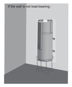
It is mandatory to install the water heater on a support . Place the water heater on the bracket to mark the fixing points.
