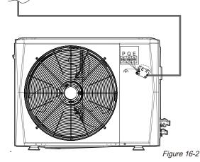
The wiring layout consists of connection cables between ODUs and IDUs (including VRF IDUs, DHW kits and hydraulic modules). It includes the IDU grounding wire and shielding layer in the communication wiring. The ODU Wiring Diagram is shown below.
