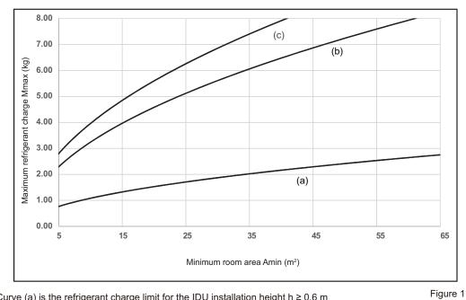
Curve (a) is the refrigerant charge limit for the IDU installation height  $h \ge 0.6$  m Curve (b) is the refrigerant charge limit for the IDU installation height 1.8 m  $\le$  h < 2.2 m Curve (c) is the refrigerant charge limit for the IDU installation height  $h \ge 2.2$  m
