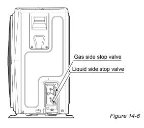
The connection method of flaring (12/14/16 kW)
