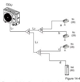
The example below illustrates the piping selection procedure for a system consisting of 1 ODU (8 kW) and 4 IDUs (3 VRF IDUs ( $2.8 \text{ kW} \times 3$ ) and 1 hydraulic module ( $8.0 \text{ kW} \times 1$ )), as shown in Figure 14-4.
