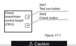
Operate the switch and button with an insulation rod (such as a ball pen with a cap) or wearing insulation gloves to avoid the contact with energized parts.
