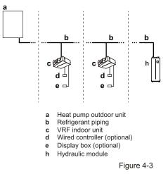
Case 4: ODU is individually connected with hydraulic module
