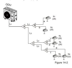
The example below illustrates the piping selection procedure for a system consisting of 1 ODU (16 kW) and 6 IDUs (2.2 kW × 1 + 2.8 kW × 5), as shown in Figure 14-2. The system's total equivalent piping length for all liquid and gas pipes is not more than 90 m.
