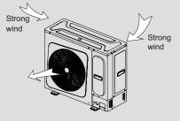
It is recommended that the fan direction of the discharge port be set at right angle to the wind direction.
