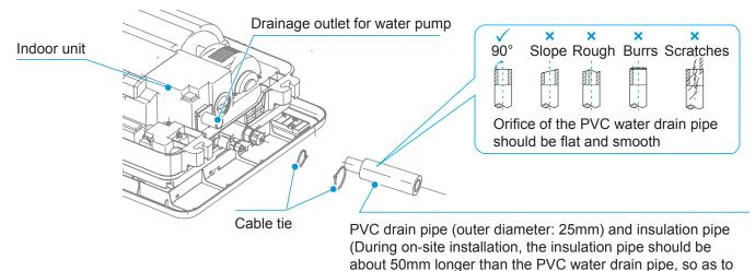
ensure that there is enough casing at the ends for insulation)
