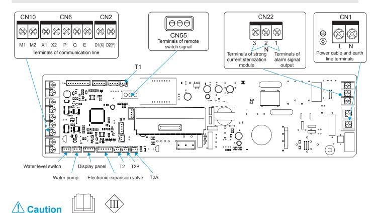
All weak point connection points meet SELV, such as X1, X2, P, Q, E, M1, M2, CN18, CN55 etc.
