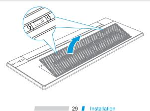
?) Toggle the buckle shown in the figure to remove the filter screen.
