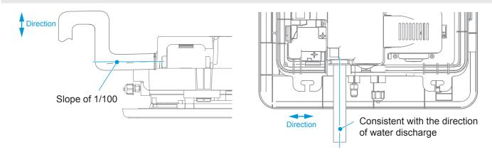
When connecting the drain pipe, do not pull the drain pipe forcefully, or it may become loose. The lateral length of the drain pipe should be within 20m, and a support point should be set every 0.8–1.0m to avoid air resistance caused by the deformation of the drain pipe. The drain pipe shall be equipped with a support point every 1.5-2.0m.
