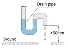
• Method to drain water with the drain pump:
