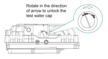
Connect the power supply, and set the air conditioner to operate in cooling mode. Check the running sound of the drain pump, and check whether the drainage outlet is draining normally (depending on the length of the drainage pipe, it may be delayed for about one minute before draining), and whether there is water leakage at each joint.
