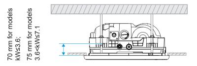
Hook the nut of the lifting bolt into the U-shaped groove of the lifting lugs. Secure the top and bottom of the lugs with washers and nuts.
