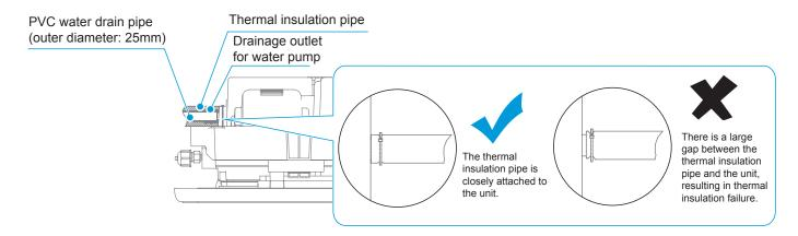
The water pump connecting pipe and drain pipe (in the indoor part) must be wrapped with heat insulation pipe evenly and bound with cable ties to prevent air from entering and producing condensate.
