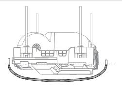
Use a transparent hose to observe water level (principle of communicating vessels) and verify the tilt angle of the unit in the length direction. It shall be installed level or at an angle within 1° towards the drainage side. (For units without a drain pump, ensure a slope of 1/100 towards the drainage side. Do not tilt towards the non-drainage side.) Otherwise, water cannot drain smoothly and leaks can easily occur.
