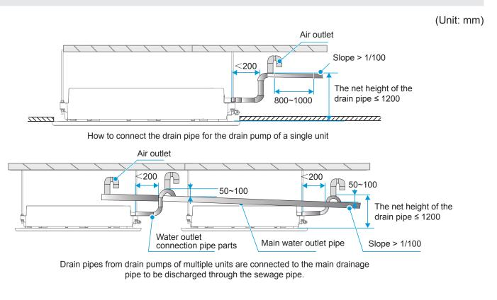
• Hedging must be prevented for horizontal drain pipes to avoid adverse slopes and poor drainage.
