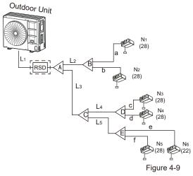
The example below illustrates the piping selection procedure for a system consisting of an outdoor unit (16kW) and 6 indoor units (2.2 kW×1+2.8 kW×5), as shown in Figure 4-9. The equivalent piping length from the outdoor units to the farthest indoor unit is not more than 90 m
