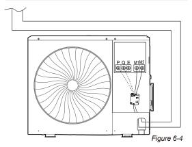
Wiring layout is comprised of the communication wiring between the indoor and outdoor units. These include the earth lines, and the shielded layer of the earth lines of the indoor units in the communication line. See below the wiring layout of outdoor unit.
