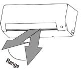
**NOTE:** Do not move louver by hand. This will cause the louver to become out of sync. If this occurs, turn off the unit and unplug it for a few seconds, then restart the unit. This will reset the buyer.
