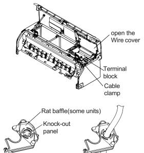
**NOTE:** If the size of the cable is too big, remove the middle small plastic knock-out panel to create a slot through which the cable can exit. If you want to remove the chassis or drain hose, please remove the rat baffle first.
