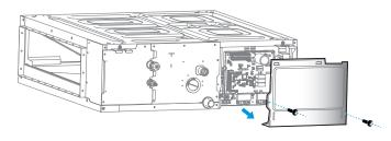
Remove the pipe clamp board.
