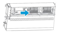
Remove the wind wheel, connecting shaft and coupling together.
