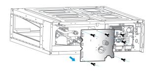
Replace temperature sensor and electronic expansion valve.
