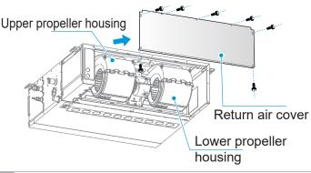
Remove the two screws from the top cover and rotate the portion of the top cover that covers the propeller housing by approximately 30 degrees around the long U-shaped hole, as shown in the figure.
