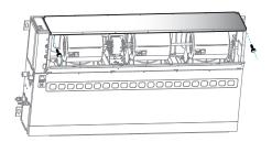
Refer to the maintenance procedure of propeller housing to remove the lower propeller housing located at the side with a coupling and loosen the fastening screws on the coupling.
