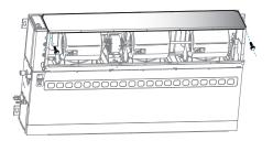
Refer to the maintenance procedure of the propeller housing to remove the lower propeller housing near the bearing block.
