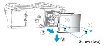
Connect the strong current wires (power cable, alarm signal output wire, and strong current sterilization wire) and weak current wires (communication line, display box connection wire, remote switch connection wire, function expansion board connection wire) to the electric control box through the bottom of the electric control box, and the strong and weak current inlets.
