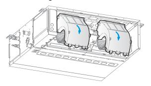
Note: Installation notes are as follows: The slot and latch bolt, and the limiting groove and side wall edge should be aligned first, and then be fastened; Check whether the limiting groove, positioning rod and buckle are installed in place, and the limiting latch bolt shall enclose the outside of the propeller housing.
