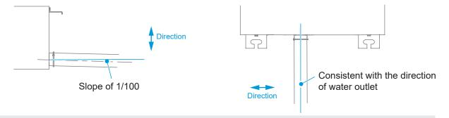
When connecting the drainage pipe, do not pull the drainage pipe forcefully, or it may become loose.
