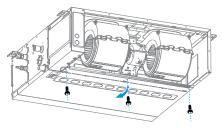
Remove the lower propeller housing in a downward diagonal direction.
