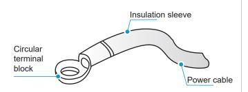
If it fails to crimp the insulated circular terminal block due to on-site limitations, connect the power cables of the same diameter to both sides of the power supply terminal block of the IDU, as shown in the figure below.
