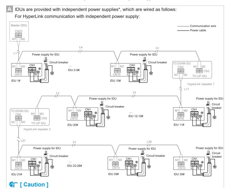
When the IDUs are provided with independent power supplies, the IDUs in the same refrigerant system should be V8 IDUs\*, and the communication between IDUs and ODU adopts a HyperLink with an independent power supply.
