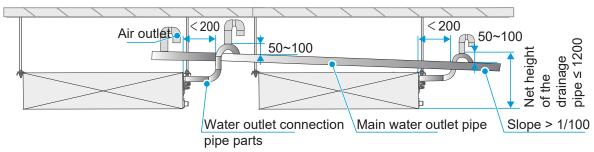
Drainage pipes from drain pumps of multiple units are connected to the main drainage pipe to be discharged through the sewage pipe.
