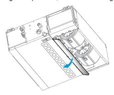
Press the buckle of the upper propeller housing, and rotate the lower propeller housing around the front edge of the lower propeller housing by about 30 degrees.
