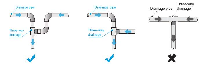
• How to discharge water without the drain pump:
