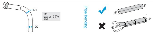
Note: D1 is the minimum diameter, and D2 is the nominal diameter.
