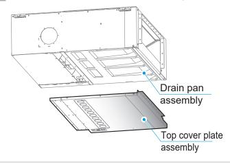
2 Remove the drain pan assembly in a downward
