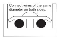
Do not press the power cables of the same wire diameter on the same side of the terminal. Do not use two power cables of different wire diameters for the same terminal blocks; otherwise, they can easily loosen due to uneven pressure and cause accidents, as shown in the figure below.
