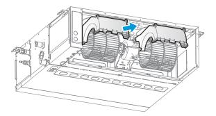
Remove the lower propeller housing in a backward direction.
