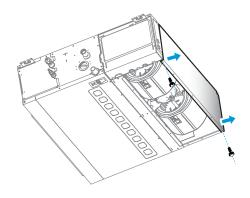
Rotate the portion of the top cover that covers the propeller housing by approximately 30 degrees around the long U-shaped hole, as shown in the figure.
