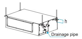
Slot the lifting bolts in the oblong holes of the lifting lugs. Secure the top and bottom of lugs with washers and nuts.
