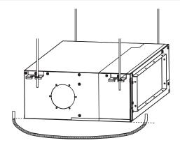
Use a transparent hose to observe water level (principle of communicating vessels) and verify the tilt angle of the unit body in the length direction, ensuring a downward slope of 1/100 towards the drainage side. Do not tilt it towards the non-drainage side.
