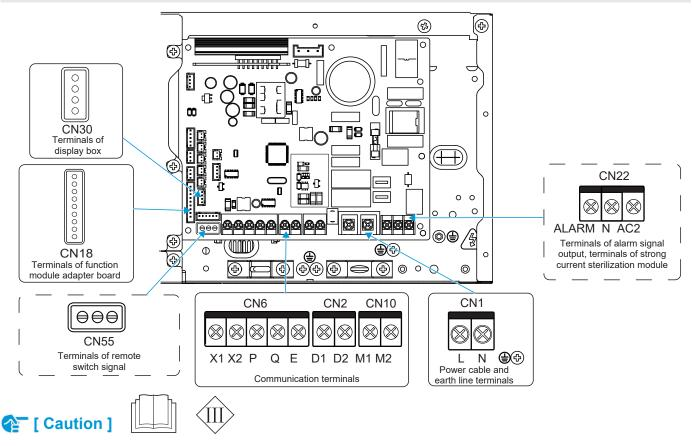
All weak point connection points meet SELV, such as X1, X2, P, Q, E, M1, M2, CN18, CN55 etc.
