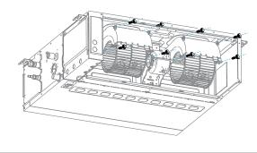
5 Move the upper propeller housing 50mm backward.
