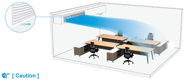
Cooling in the downward outlet state may cause condensation on the air outlet and guide louver surface.
