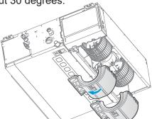
Loosen the fastening screws for the motor sealing plate and wind wheel.
