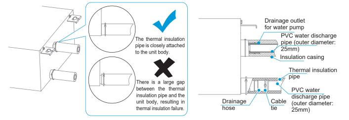
The water pump connecting pipe and drainage pipe (in the indoor part) must be wrapped with heat insulation pipe evenly and bound with cable ties to prevent air from entering and producing condensate.
