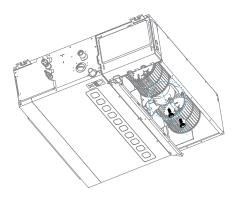
5 Remove the motor and wind wheel together.
