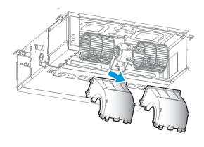
Make the propeller housing rotate more than 90° downward along the wind wheel.
