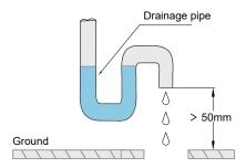
Method to discharge water with the drain pump:
