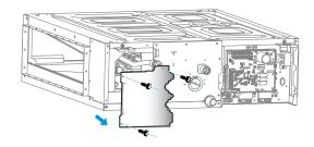
3 Remove and repair the drain pump assembly.
