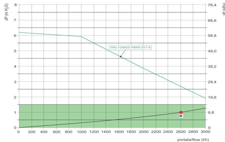
Low temperature water pump (mixed water):
