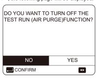
Press ◀ ► to scroll the cursor to YES and press —. The test run will turn off.
