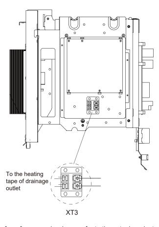
The picture is for reference only, please refer to the actual product. The power of the E-heating tape shall not exceed 40W/200mA, supply voltage 230VAC.
