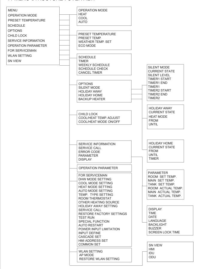
FOR SERVICEMAN 1 DHW MODE SETTING 2 COOL MODE SETTING 3 HEAT MODE SETTING 4 AUTO MODE SETTING 5 TEMP. TYPE SETTING **6 ROOM THERMOSTAT** 7 OTHER HEATING SOURECE 8 HOLIDAY AWAY SETTING 9 SERVICE CALL 10 RESTORE FACTORY SETTINGS 11TEST RUN 12 SPECIAL FUNCTION 13 AUTO RESTART 14 POWER INPUT LIMITATION 15 INPUT DEFINE 16 CASCADE SET 17 HMI ADDRESS SET 18 COMMON SET
