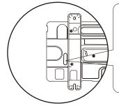
This drain hole is covered by rubber plug. If the small drain hole can not meet the drainage requirements, the big drain hole can be used at the same time.
