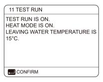
During HEAT MODE test running, the default target outlet water temperature is 35°C. The IBH (backup heater) will turn on after the compressor runs for 10 min. After the IBH runs for 3 minutes, the IBH will turn off, the heat pump will operate until the water temperature increase to a certain value or the next command is received.
