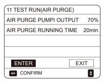
Press ▼ ▲ ◀► to adjust the parameters, click "ENTER" to send the setting parameters, the following pages will be displayed:
