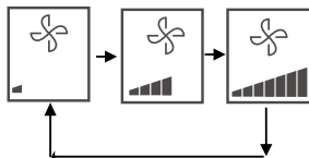
Fig. 28 The sequence of 3 fan speeds of HRV Auto Fan
