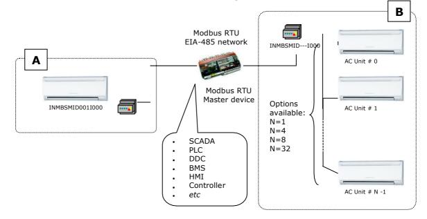
A Integration of single AC unit from independent XYE bus using INMBSMID001I000 interface
