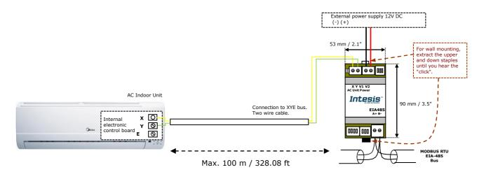
Figure 2.1 INMBSMID001I000 connection diagram
