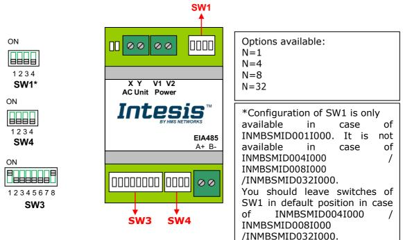
The following tables apply to the interface's configuration through DIP-switches:
