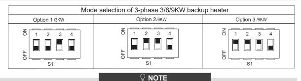
The default of backup heater is as option 3 (for 9kW backup heater). If 3kW or 6kW backup heater is needed, please ask professional installer to change the Dip switwch S1 to option 1(for 3kW backup heater) or option 2(for 6kW backup heater), refer to 9.2.1 FUNCTION SETTING.
