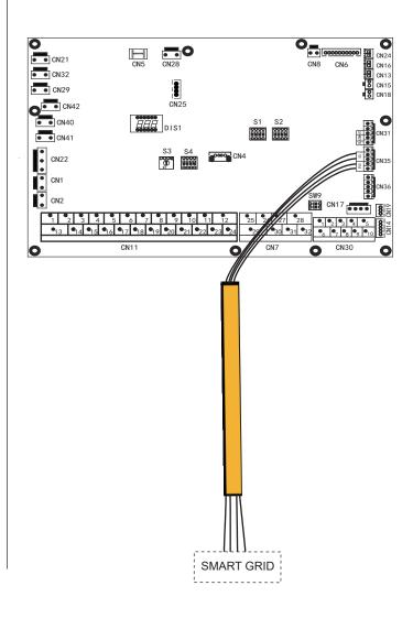
1. When EVU signal is on , and SG signal is on, as long as the DHW mode is set to be valid, heat pump will operate DHW mode priority and the DHW mode setting temperature will be change to 70 °C . T5<69 °C , the TBH is on,T5≥70 °C , the TBH is off.
