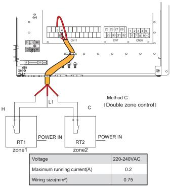
There are three methods for connecting the thermostat cable (as described in the picture above) and it depends on the application.
