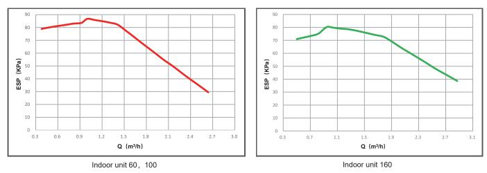
Available external static pressure VS Flow rate Available external static pressure VS Flow rate
