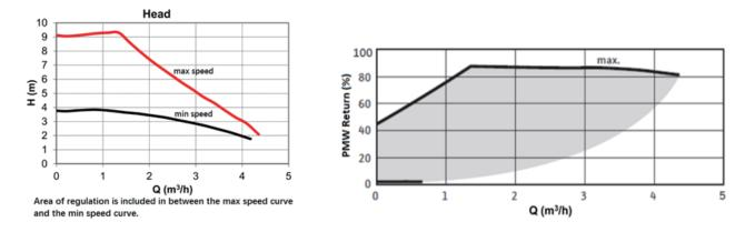
The internal pump maintains maximum output, the indoor unit can provide the head and flow:
