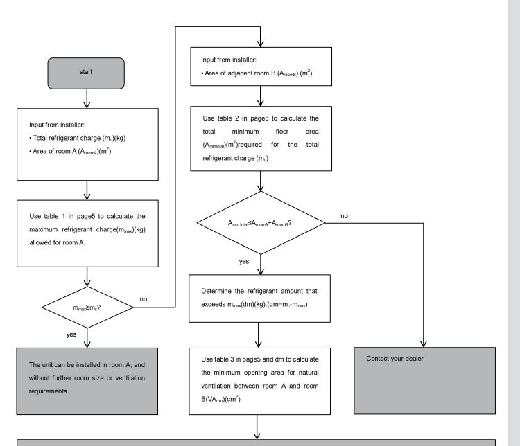
Unit can be installed at room A if:
