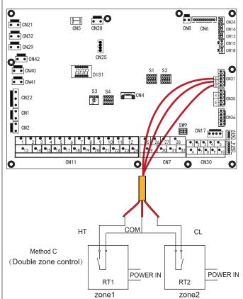
There are three methods for connecting the thermostat cable (as described in the picture above) and it depends on the application.
