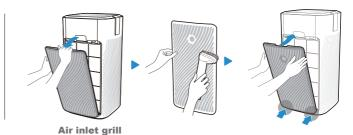
Open the air inlet grill, clean dust with a vacuum cleaner, and wipe it with a cloth.
