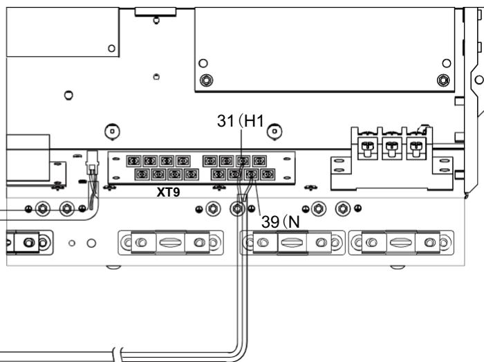
Fix the cable with cable ties to the cable tie mountings.
