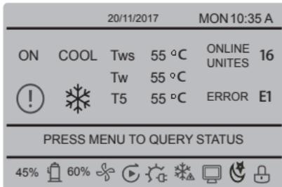
When the wired controller is unlocked, press "MENU" button to enter the "SERVICE MENU" function.
