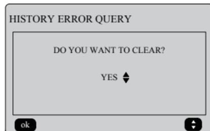
Press the "▼" and "▲" buttons to select the desired option, If "YES" is selected then press the "OK" button to clear current address error, and return to the "HISTORY ERROR QUERY" interface. If "NO" is selected then press "OK" button to return to the "HISTORY ERROR QUERY" interface directly.
