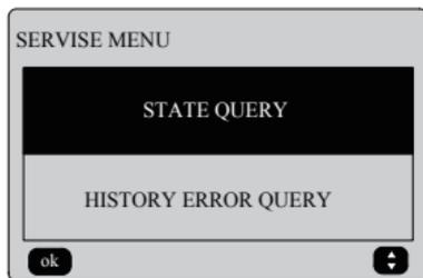
Press the "▼" and "▲" buttons to select the desired option, and press the "OK" button to access the interface. Press the "BACK" button to cancel the setting and return to the previous interface.
