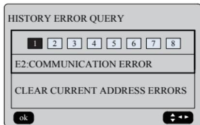
Press the "◀" and "▶" buttons to view records of error history, press "OK" button back to "HISTORY ERROR QUERY" interface. Press "▼" and "▲" buttons to select "CLEAR CURRENT ADDRESS ERRORS" and press "OK" button to clear current address error, and enter the interface, the interface is as follows:
