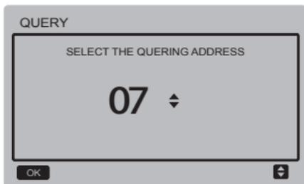
Press the "▼" and "▲" buttons to select the address of module to view (the offline address is skipped automatically). Press the "OK" button to access the lower-layer submenu, or press "BACK" to go back to the previous interface. During operation on the menu page, press "BACK" to go back to the previous interface. if there is no operation in 60 seconds, the wired remote controller will return to the home page. If there is no error, press the "OK" button will enter the interface as follows:
