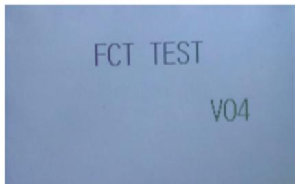
After entering the page displays the version number, All parameters are reset to the default parameters, and eliminate time setting and the fault records. The equipment back to the factory at the same time. To exit the FCT function should power on again.
