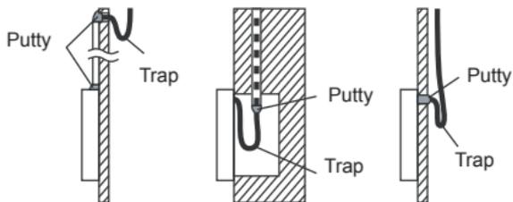
Avoid the water enter into the wired remote controller, use trap and putty to seal the connectors of wires during wiring installation.
