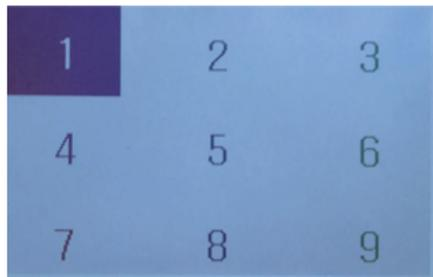
Press "MENU" → "▲" → "ON/OFF" → "◀" → "OK" → "▶" → "BACK" → "▼" → "UNLOCK" buttons one by one to light 1-9 to enter the FCT interface. The interface display is as follows:
