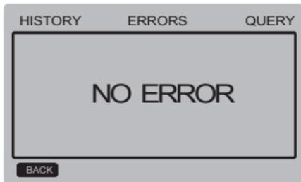
The wired controller can display 8 errors at most. Take the mainboard (00#) as an example to make further explanation of the submenu. After the mainboard is selected, the running state of mainboard is as shown below:
