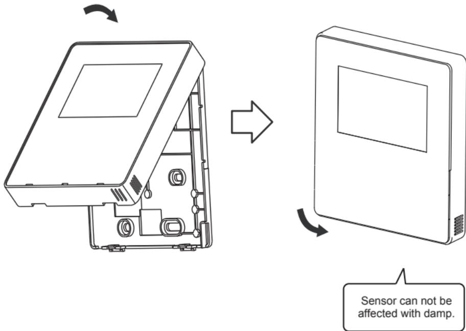
Correct install the back cover and firmly buckle the front cover and back cover, otherwise will make the front cover drop off.
