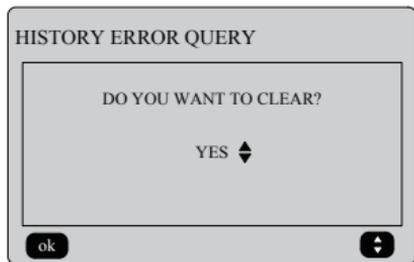
Press the "▼" and "▲" buttons to select the desired option, If "YES" is selected then press the "OK" button to clear all history errors, and return to the "HISTORY ERROR QUERY" interface. If "NO" is selected then press "OK" button to return to the "HISTORY ERROR QUERY" interface directly.
