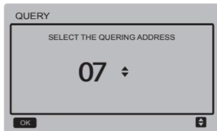
Press the "▼" and "▲" buttons to select the address of module to view (the offline address is skipped automatically). Press the "OK" button to access the lower-layer submenu, or press "BACK" to go back to the previous interface. During operation on the menu page, press "BACK" to go back to the previous interface. if there is no operation in 60 seconds, the wired remote controller will return to the home page.
