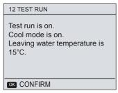
During COOL MODE test running, the default target outlet water temperature is 7°C, the unit will operate until the water temperature drop to a certain value or the next command recived.
