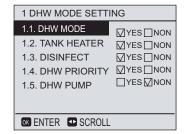
Use ◀ ▶ to scroll and OK for enter. When the cursor is on ☐ YES, Press OK to set the DHW MODE as effective.
