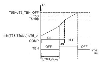
In the picture, T5stop is a parameter related to ambient temperature, which cannot be changed in the user interface. When T5≥T5stop, the heat pump will turn off.
