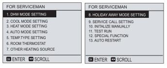
Use  $\P$   $\blacktriangle$  to scroll and use "ok" to enter submenu for setting the parameters.
