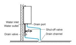
When water is at standstill inside the system, freezing is very likely to happen and damaging the system in the process.
