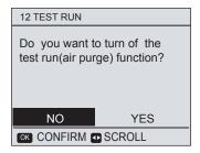
Using  $\blacktriangleleft$ ,  $\blacktriangleright$  to scroll the cursor to YES and press OK, the test run will turn off.
