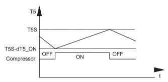
T5S is the target temperature for domestic hot water. T5 is the actual temperature of domestic hot water. When T5 drops to a certain temperature (T5≤T5S-dT5\_ON) the heat pump will be available. dT1S5 is the correct value for the target outlet water temperature (T1S=T5+dT1S5).
