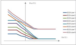
High temperature curves for heating ECO mode
