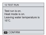
During HEAT MODE test running, the default target outlet water temperature is 35°C, the first backup heater will turn on after the compressor runned for 10min, 60s later the second backup heater will turn on. After the two backup heater runned for 3min, both backup heater will turn off, the heat pump will operate until the water temperature increase to a certain value or the next command recived.
