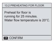
During preheating for floor, all the buttons except OK is invalid. If you want to turn off the preheating for floor, please press OK, then the page will displayed as following:
