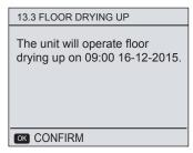
During floor drying up, all the buttons except OK is invalid. When the heat pump malfunction, the floor drying mode will turn off when the backup heater and additional heating source is unavailable. If you want to turn off the floor drying up, please press OK, then the page will displayed as following:
