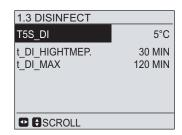
T5S\_DI is the target temperature of water in the domestic hot water tank in the DISINFECT function.
