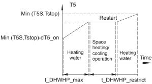
If NON is selected in the DHW PRIORITY mode, when it is available and the space heating/cooling is OFF, the heat pump will heat the domestic water as required. If space heating/cooling is ON, the domestic water will be heated by booster heater(if booster heater is available).
