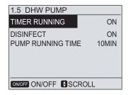
When the **TIMER RUNNING** is **ON**, the DHW pump will run as timed and keeps running for an certain time (as defined in **PUMP RUNNING TIME**), this can ensure the temperature of water in the system are uniform.
