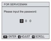
The password is 666. Use ◀ ► to navigate and use ▼ ▲ to adjust the numerical value. Press OK. The following page is displayed:
