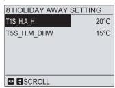
When the cursor is on T1S\_H.A.\_H or T5S\_H.M\_DHW, Use ◀ ▶ and ▼ ▲ to scroll and adjust the parameter, T1S\_H.A.\_H is the target outlet water temperature for space heating when in holiday away mode. T5S\_H.M\_DHW is the target outlet water temperature for domestic hot water heating when in holiday away mode.
