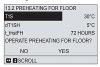
When the cursor is on T1S, dT1SH or t\_fristFH, Using  $\blacktriangleleft$ ,  $\blacktriangleright$ ,  $\blacktriangledown$ ,  $\blacktriangle$  to scroll and adjust the parameter.
