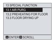
Use ▼, ▲ to scroll and use OK to enter. During first operation of the unit, air may remained in the system which can case malfunction during operation, so it is necessary to run air purge function to release the air(make sure the air purge value opened).
