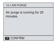
During air purge, the 3-way value will open, the 2-way value will close, 60seconds later the pump in the unit(PUMPI) will operate for 10min, during which the flow switch will not work. after the pump stoped, the 3-way value will close and the 2-way value will open, 60s later the both the PUMPI and PUMPO will operate until the stopping command recived
