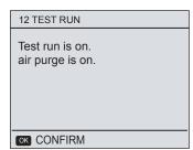
When in air purge mode, the 3-way value will open, the 2-way value will close, 60s later the pump in the unit(PUMPI) will operate for 10min, during which the flow switch will not work. after the pump stoped, the 3-way value will close and the 2-way value will open, 60s later both the PUMPI and PUMPO will operate until the next command recived.
