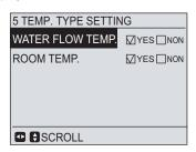
If you set WATER FLOW TEMP. to YES, and set ROOM TEMP. to NON, the water flow temperature will be displayed on the home page, and the water flow temperature will work as the target temperature.
