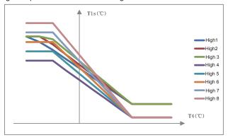
Low temperature curves for heating ECO mode
