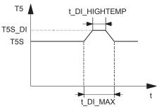
Be aware that the domestic hot water temperature at the hot water tap will be equal to the value selected in FOR SERVICEMAN "T5S\_DI" after a disinfection operation.
