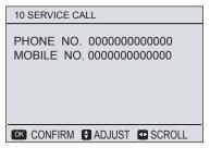
Using ▼, ▲ to scroll and set the phone number, the maxmuim length of the phone number is 13, if the length of phone number short than 12, please input ■, as described in the picture below:
