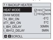
When the cursor is on HEAT MODE or DHW MODE, Use ◀ ▶ to select YES or NON. If YES is selected, the backup heater will be available in the corresponding mode, otherwise it will be unavailable.
