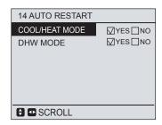
Use ▼, ▲, ◄, ► to scroll and use OK to select YES or NON to enable or disable the auto restart function. If the auto restart function is enabled, when power returns after a power supply failure, the AUTO RESTART function reapplies the user interface settings at the time of the power supply failure. If this function is disabled, when power returns after a power supply failure, the unit won't auto restart.
