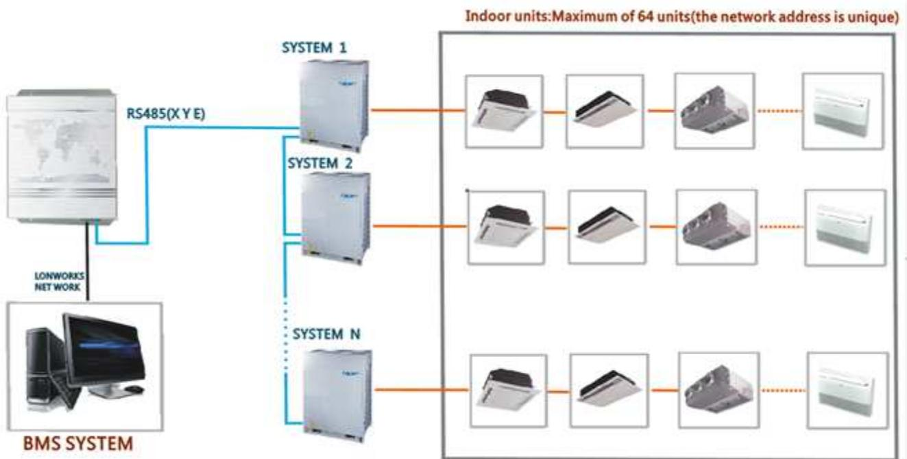
**Notes:** If there are a few K01-Lon devices to compose a LonWorks network, the LonWorks terminals of the K01-Lon are able to be connected in the hand-in-hand way. And can be connected up to 64 indoor units to the LonWorks network.
