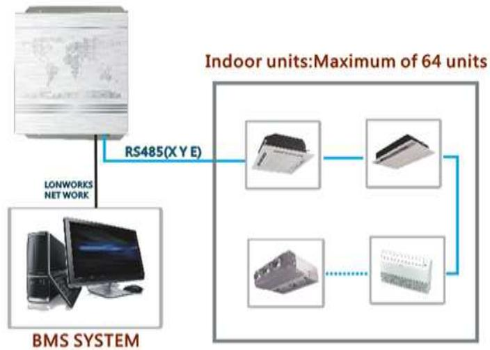
This connection method is suitable for all of the air conditioners system.
