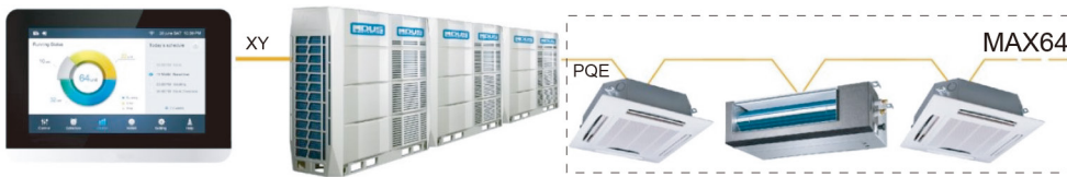
Fig-1(a) Controller to Single Outdoor Unit Wiring Diagram
