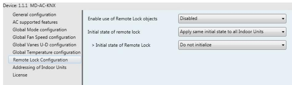
Figure 4.24 Parameter detail
