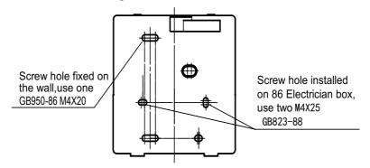
4) Adjust the length of two plastic screw bars in the accessory to be the standard length from the electrical box screw bar to the wall. Make sure when install the screw bar to the electrical box screw bar, make it as flat as the wall.
