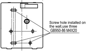
3) Use two M4X25 GB823-88screws to install the back cover on the 86 electrician box, and use one GB950-86 M4X20 screw for fixing the wall.
