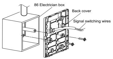
**Notes:** 1.Use cross head screws to fix the wired controller bottom cover in the electric control box through the screw bar. Make sure the wired controller bottom cover is on the same level after installation, and then install the wired controller back to the bottom cover.
